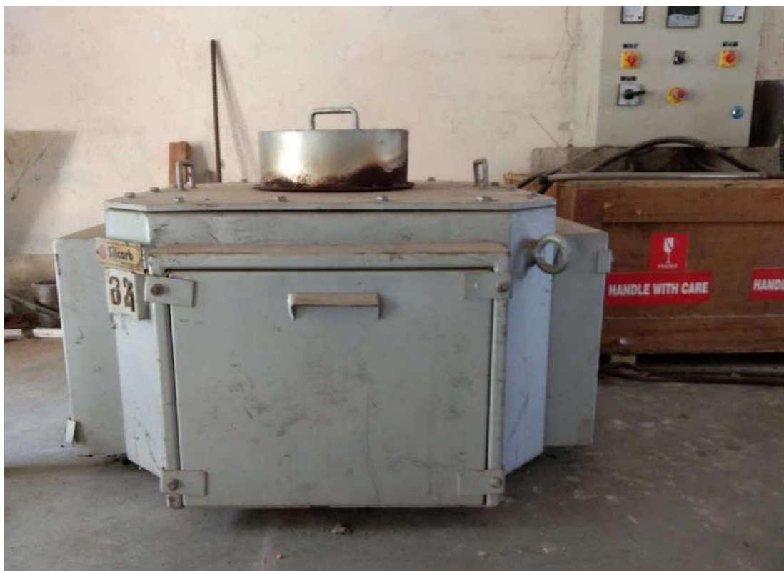
Fig.1 Electric resistance furnace with control unit.
