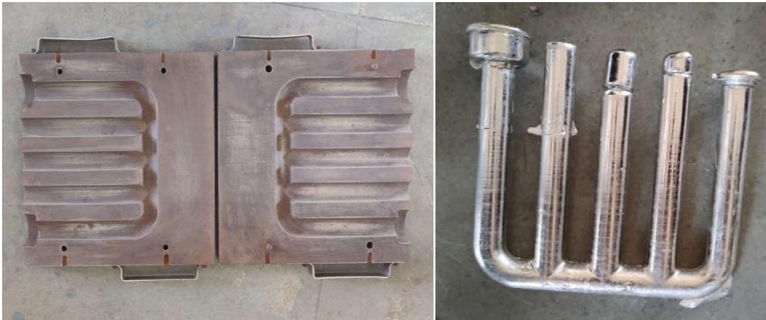
Fig.2 (a) Metallic Die (b) Casting after solidification
