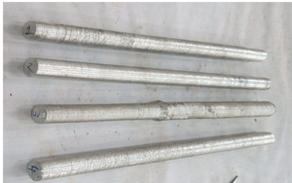
Figure6: Before Tensile test image
