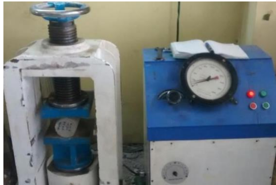
Fig -2: Split tensile Strength – Experimental set up
